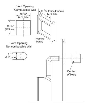
Figure 9 - Vent Opening Requirements
